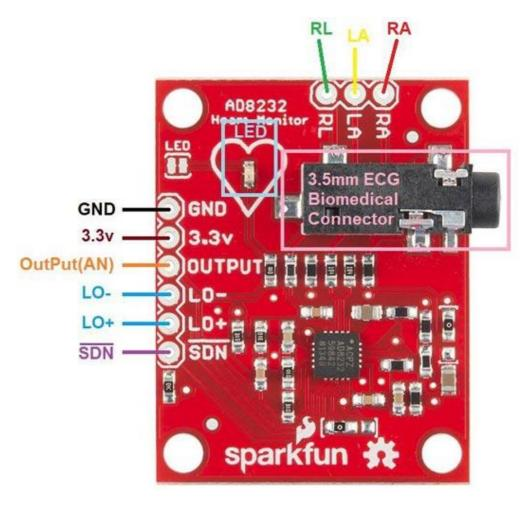
AD8232 ECG Module integrated with AD8232 IC from Analog Devices, which is a single-chip designed to extract, amplify, and filter biopotential signals for biopotential measurement applications (like ECG and others). ECGs can be extremely noisy so that the AD8232 Single Lead Heart Rate Monitor acts as an op-amp to help obtain a clear signal from the PR and QT Intervals easily.
