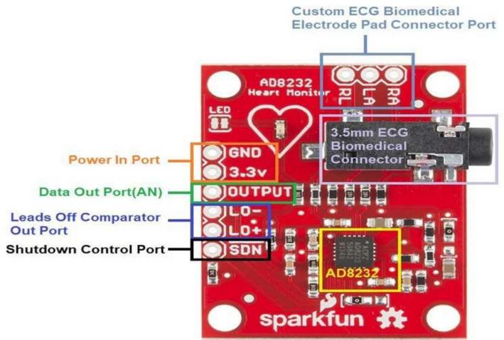
The AD8232 ECG Module is a cost-effective board used to measure the electrical activity of the heart. This electrical activity can be charted as an ECG or Electrocardiogram and output as an analog reading.
